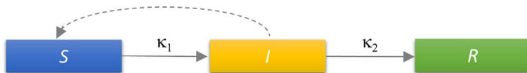
Fig. 2 Schematic representation of the SIR model. Rectangles denote model compartments containing susceptible ( S ), infected ( I ), and recovered ( R ) individuals in the population of size N . Permitted directions of flow between compartments are denoted by arrows, with the rates of flow indicated above them. The rates are expressed according to the law of mass action, where \kappa_1 and \kappa_2 are the rate constants. The dashed curve corresponds to bimolecular reaction, where newly infected are generated through interactions (contacts) between susceptible and already infected individuals.
